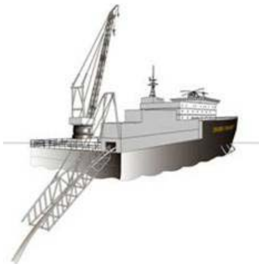
Illustration: Pipe lay barge
