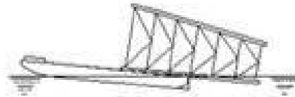
Moving jacket along skid beams Step 2
